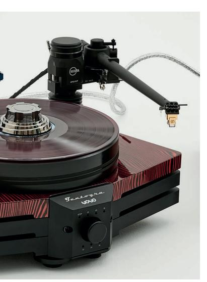
The Tentogra WoWo has a very favourable centre of gravity distribution. I used a DC motor like in the Oscar model to drive the platter. Each of the speeds of 33, 45 and 78 RPM is activated by a knob on the front of the turntable. The current speed is indicated by the appropriate LED on the turntable front. The motor is an independent object, not coupled with the structure so as not to transfer vibrations to the plinth. One can also use a battery of my production, which is not standard equipment.
